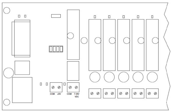
Figure 6: Power Supply Terminal Blocks
