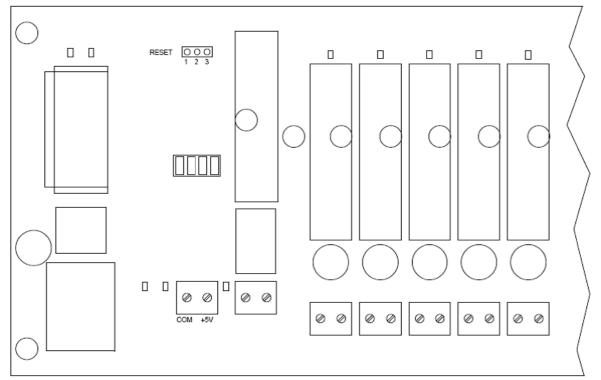
Figure 1: Reset Jumper Location
